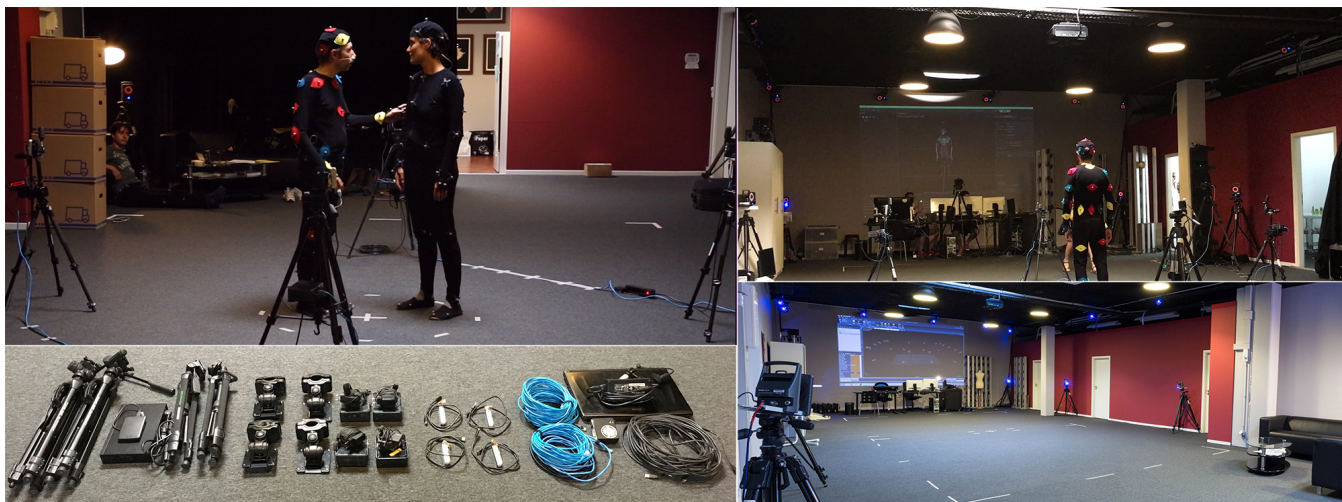
FIGURE 1: Pictures taken during the preparation and capturing of the HUMAN4D dataset (in Artanim’s facilities). The room is equipped with 24 Vicon MXT40S cameras rigidly placed on the walls, a portable volumetric capturing system with 4 Intel RealSense D415 depth sensors temporarily set up to capture the RGBD data cues and wearable microphones for the actors.
